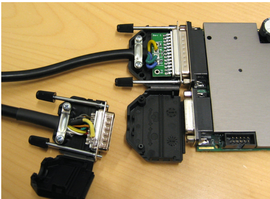
Figure 3: Wired encoder & motor D-sub connectors (covers opened)
