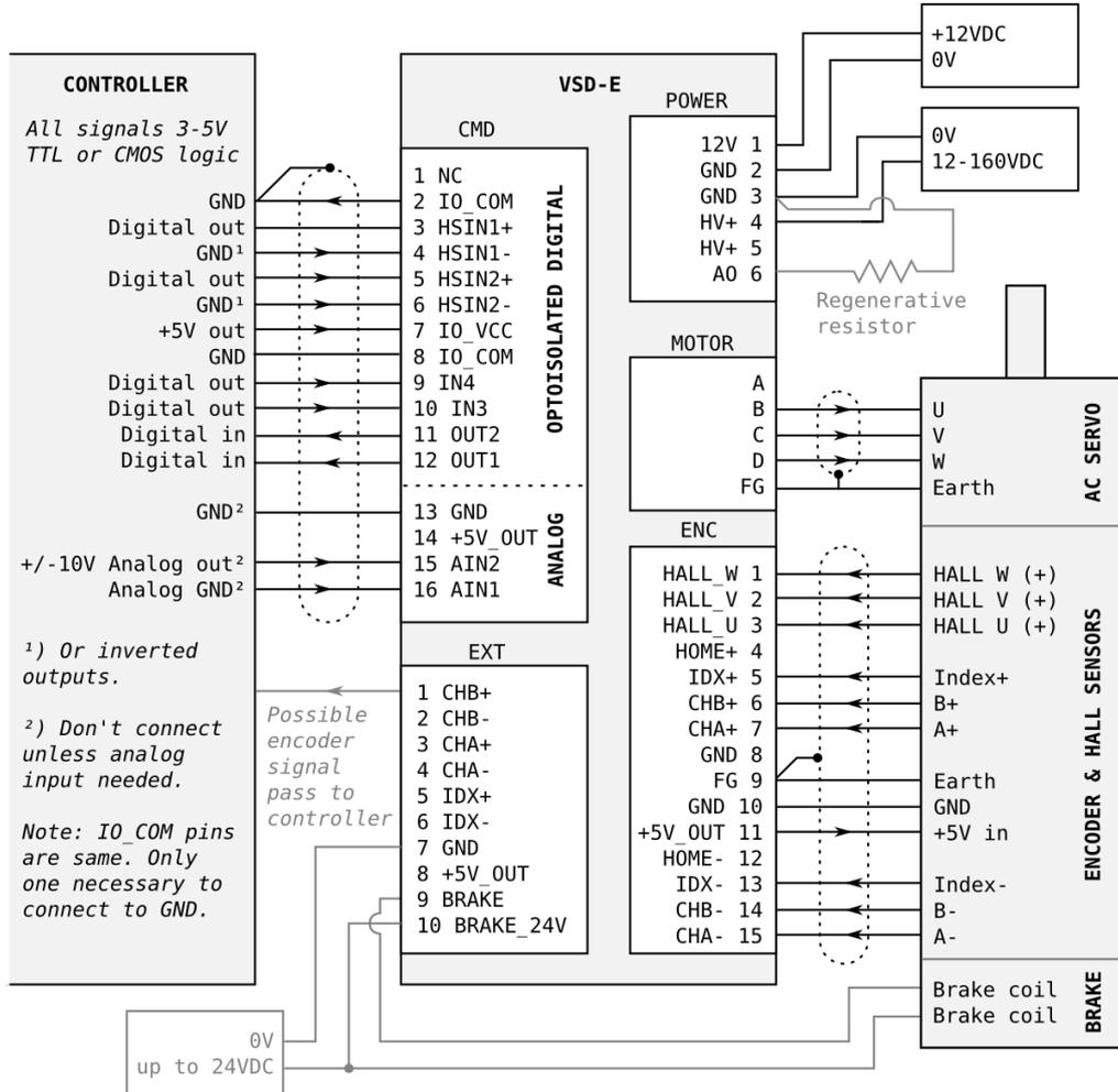
Figure 13: Typical controller and motor wiring. This example uses AC motor with Hall sensors and holding brake. All of connections are not needed if certain features are not used.
