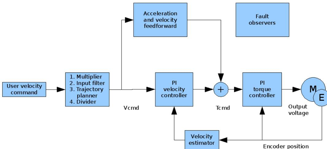
Figure 16: Overview block diagram of PI type velocity controller.
