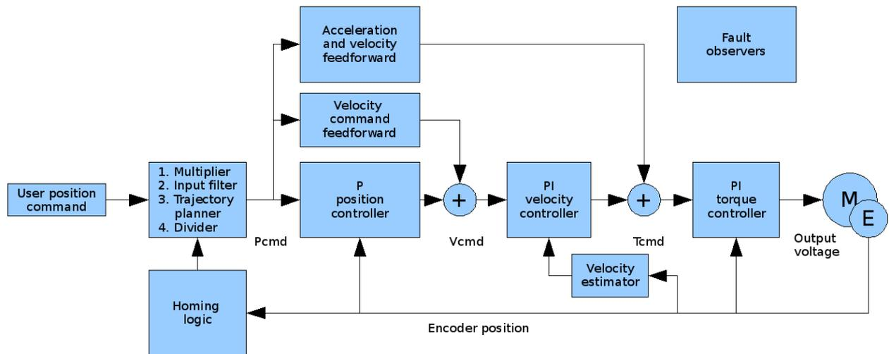
Figure 17: Overview block diagram of PIV type position controller.
