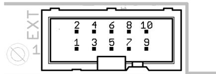
Figure 11: EXT connector (5x2 0.1" centers shrouded header)
