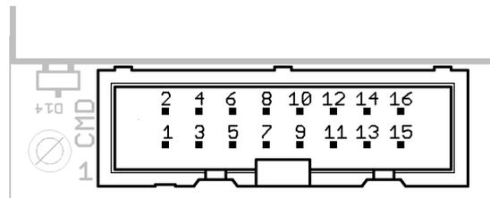
Figure 7: CMD connector (8x2 0.1" centers shrouded header)
