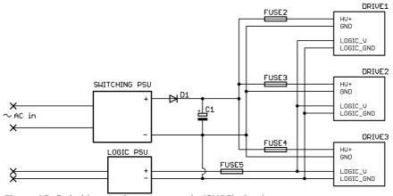
Figure 15: Switching mode power supply (SMPS) circuit
