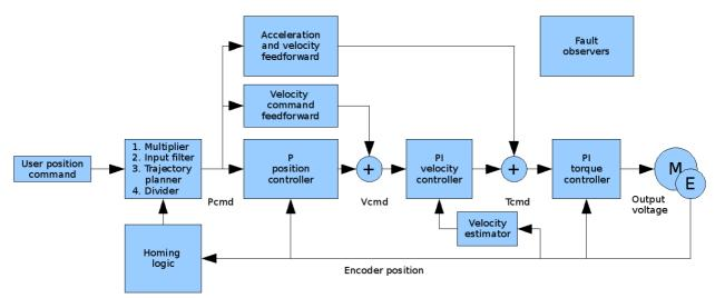
Figure 17: Overview block diagram of PIV type position controller.
