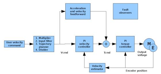
*Figure 16: Overview block diagram of PI type velocity controller.*
