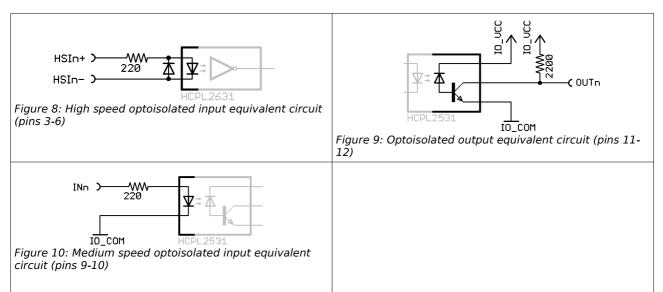
Note: In the schematics figures the shaded end represents drive logic side, which is insignificant from user's point of view.
