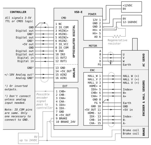
Figure 13: Typical controller and motor wiring. This example uses AC motor with Hall sensors and holding brake. All of connections are not needed if certain features are not used.
