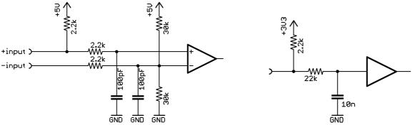
Figure 5: Equivalent circuit for differential inputs (pins 4-7 and Figure 6: Equivalent circuit for Hall sensor 12-15) inputs (pins 1-3)
