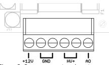
Figure 2: Power connector pin out
