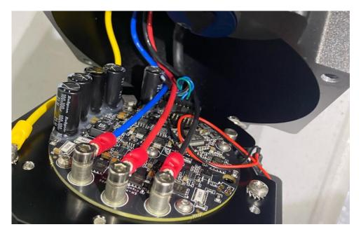
Example image of a bad PSU power cable placement which caused the device to have issues to start up.
