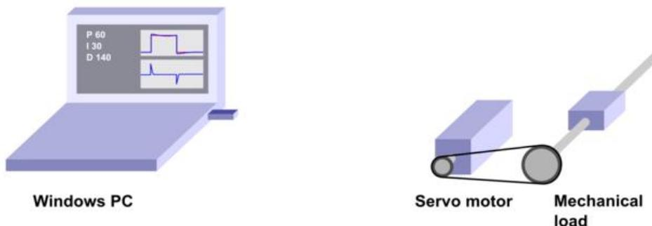
After motor and drive are fully functional, connect motor to the mechanical load and find the optimum velocity or position control gains. Read the main article [Servo motor tuning guide](#).
